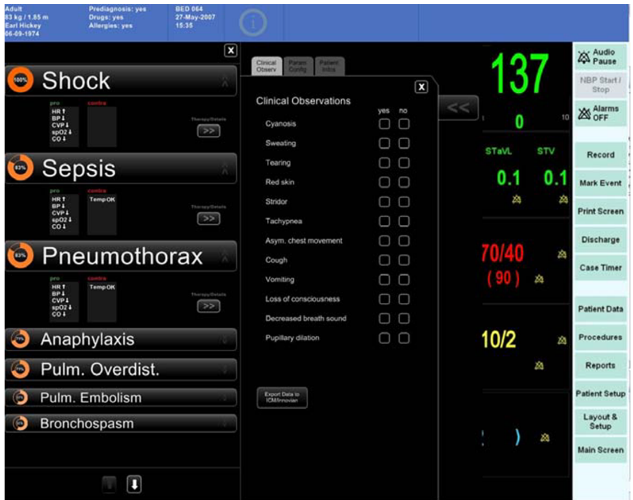
Figure 6. Diagnosis Display was developed in the study by Kindsmüller et al. (2009). Incorporated into an existing patient monitor, it provided information on the patient's state and symptoms, as well as possible diagnoses. It allowed both the option of a quick overview of all possible diagnoses, as well as the viewing of more detailed information of the symptoms these diagnoses were based on.
