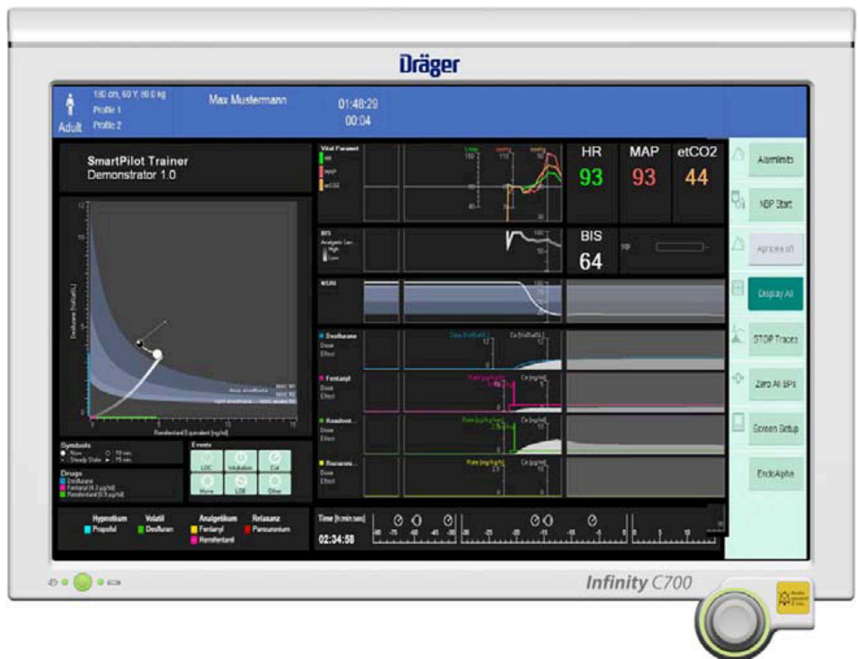
Figure 5. Smart Pilot comprehensively presented all the information which anesthesiologists needed to accurately calculate the drug dosage needed for their patients. Beforehand, anesthesiologists had needed to monitor several different devices that additionally presented various information that they had no need for. To find the information they were looking for, anesthesiologists were forced to consciously filter out all the irrelevant data – a distraction made unnecessary through the use of Smart Pilot (Kindsmüller et al., 2009).
